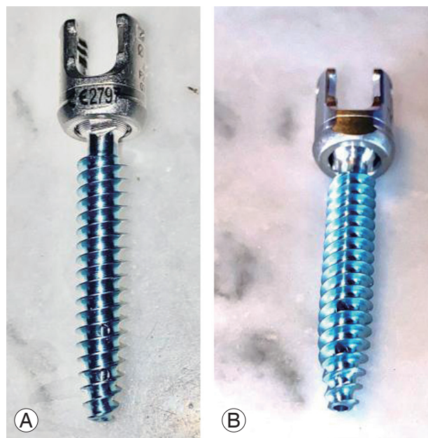
Fig. 1. (A, B) Example of a fenestrated pedicle screw demonstrating cannulated core and fenestrations for cement delivery.
