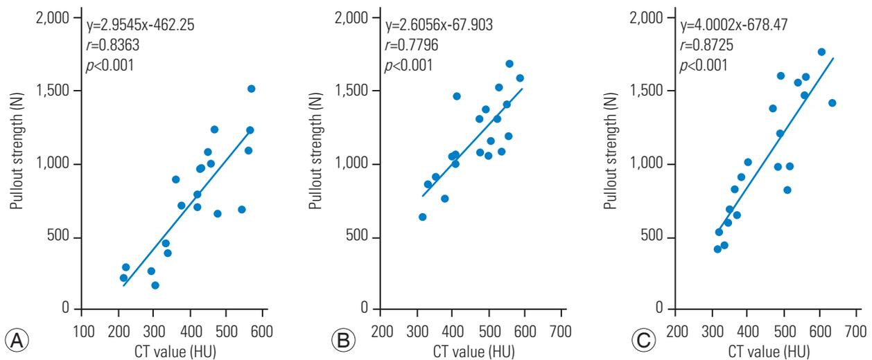
**Fig. 4.** Relationships between the CT values and pullout strengths (N) of (A) 4.0-LEG (LEGACY; diameter, 4.0 mm; length, 30 mm), (B) 4.5-LEG (LEGACY; diameter, 4.5 mm; length, 30 mm), and (C) 4.5-SOL (SOLERA; diameter, 4.5 mm; length, 30 mm) screws. The CT values were significantly positively correlated with the pullout strengths (N) of all pedicle screws ( $p < 0.001$ ). CT, computed tomography; HU, Hounsfield units.
