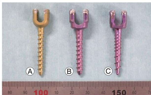
**Fig. 1.** Photographs showing the screw types used in the present study. (A) 4.0-LEG (LEGACY; diameter, 4.0 mm; length, 30 mm), (B) 4.5-LEG (LEGACY; diameter, 4.5 mm; length, 30 mm), and (C) 4.5-SOL (SOLERA; diameter, 4.5 mm; length, 30 mm).
