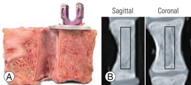
**Fig. 2.** Images of the porcine vertebrae. (A) Photograph of a 30-mm-long screw inserted through a 2-mm-thick washer. (B) Computed tomographic image showing the 10×30-mm rectangular region of interest (enclosed by the black lines); cortical margins were excluded to prevent volume averaging.
