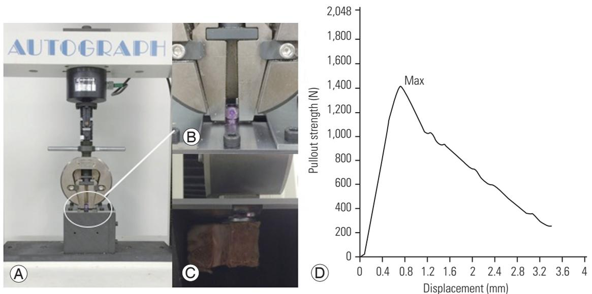
**Fig. 3.** Biomechanical testing. (A) The autograph used to determine pullout strength (N) at a displacement rate of 1.0 mm/min. (B) A screw head attached to the testing machine. (C) The bone–screw complex fixed inside the metal box. (D) Typical load–displacement curve for screw axial pullout.
